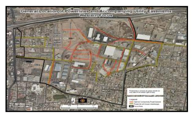
Figure 5; General Location of Power lines and Accompany Easements Western Focus
